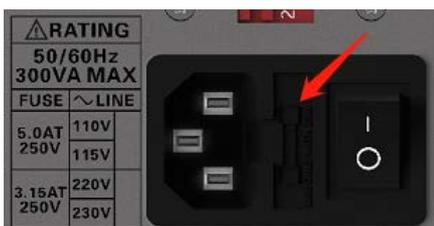
3. Remove the fuse and install a new one.
